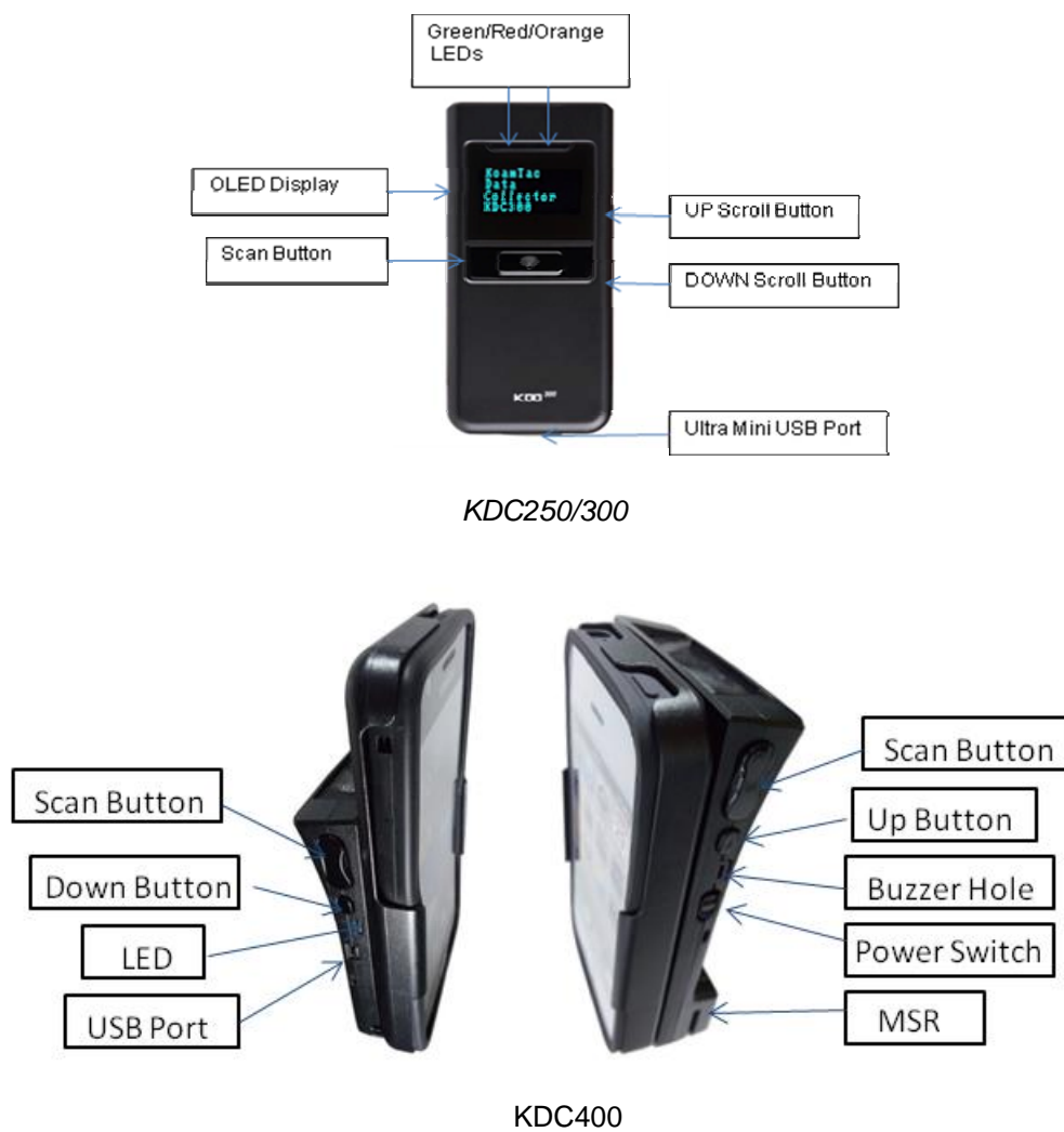
Figure 3 - Characteristics of KDC200 / KDC250 / KDC300
