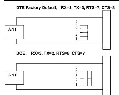
DTE 3 Wire ( (CTS shorted to RTS) , remove 3<sup>rd</sup> , 4<sup>th</sup> jumpers and install one of the removed jumpers in position 5
